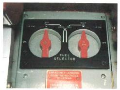
pumps are controlled by separate ON-OFF toggle switches. The fuel management system is the simplest there is. Just select ON, OFF, or CROSSFEED.
